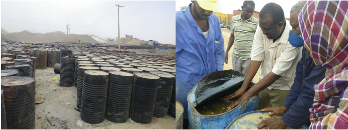
Figure 5.1 Sampling of Bitumen in J. Toria Plants
