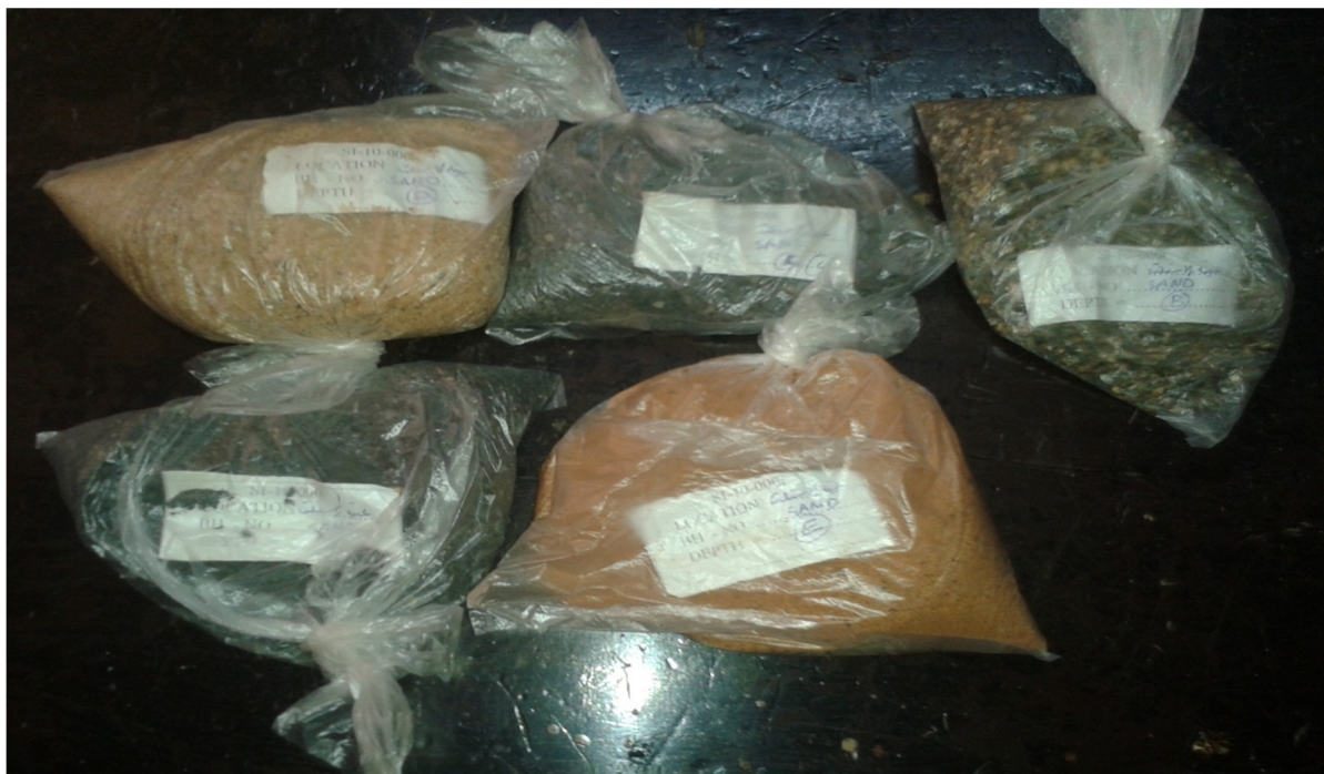
Figure 5.2: The Prepared Samples for Angularity Test
