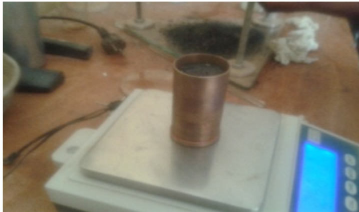
Figure 2-4: Nominal 100 Cm 3 Calibrated Cylinder Measure
