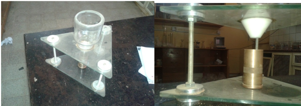
Figure 2.5: Funnel Stand Apparatus
