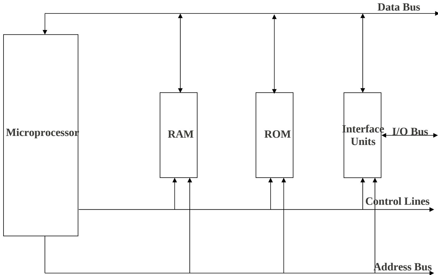
**Figure. (3.1) Microcomputer System Block Diagram**
