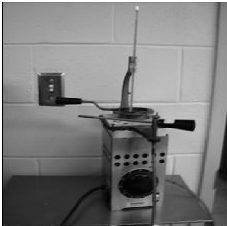
Figure 3.5: Cleveland Open Cup Flash Point
