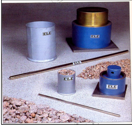
Figure 3.7: ACV apparatus & Aggregate Crushing Test Machine
