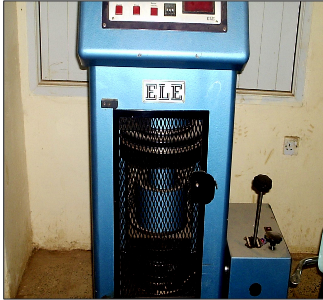
Figure 3.7: ACV apparatus & Aggregate Crushing Test Machine
