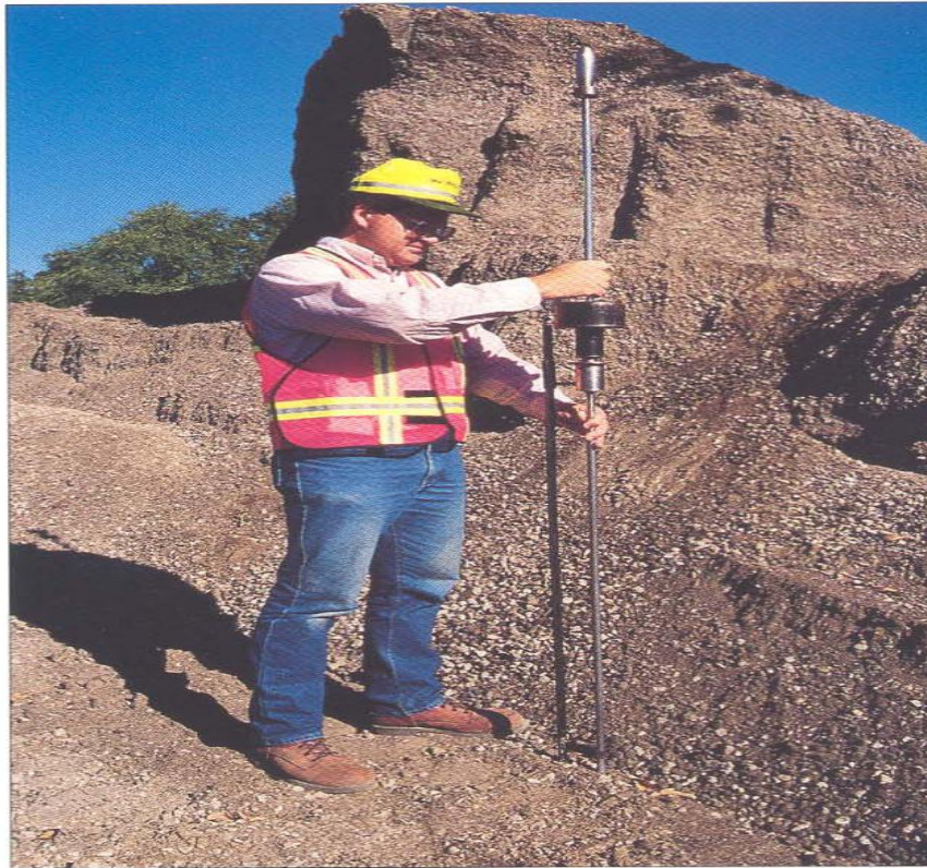
Plate (A2): Minnesota Dynamic Cone Penetrometer
