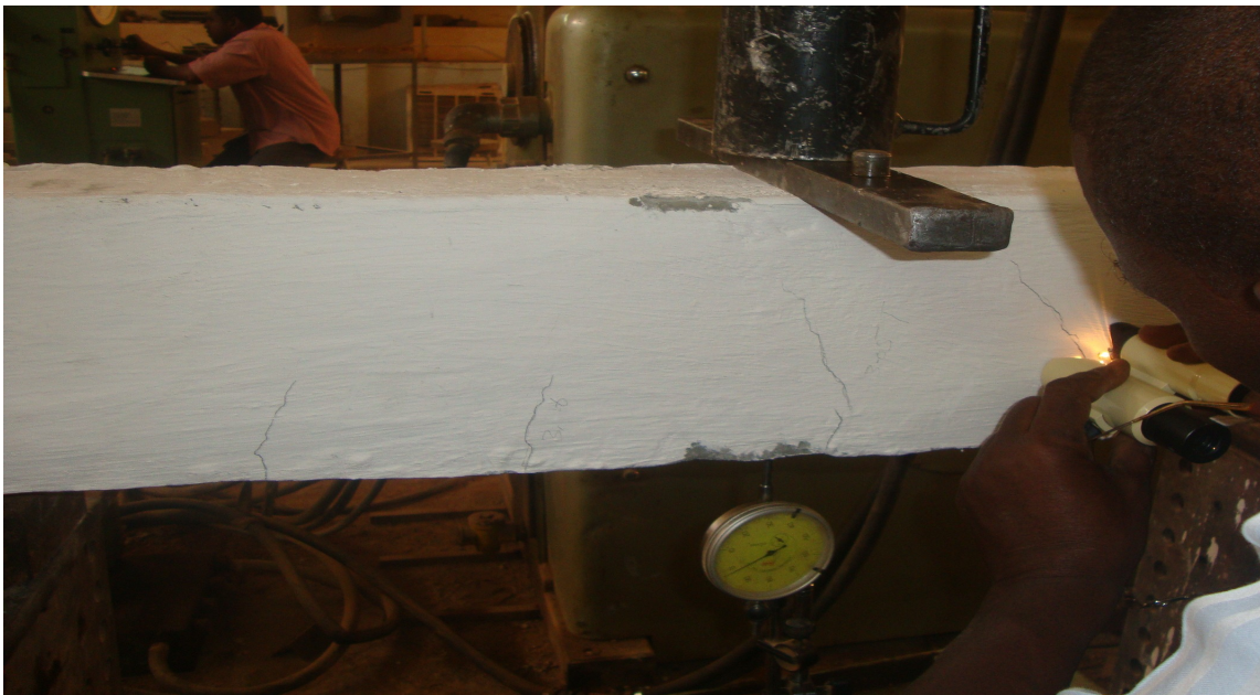
C9 - Reading First Cracking
