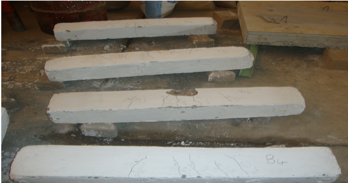
C10 - Failure Beams
