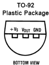
Figure A.2: LM35 Package
