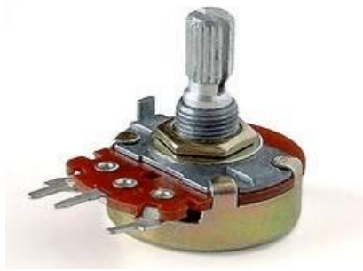
Figure 3.4: shows a typical single-turn potentiometer
