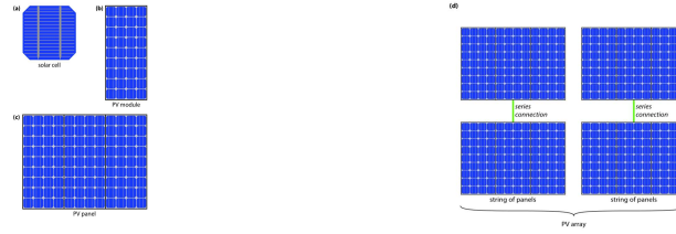
Figure (2.4): Illustrating (a) a solar cell, (b) a PV module, (c) a solar panel, and (d) a PV array.
