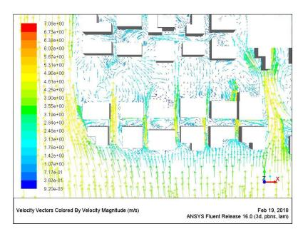
Figure 7.52 Wind pattern around buildings at a height of 1.5m [Author]
