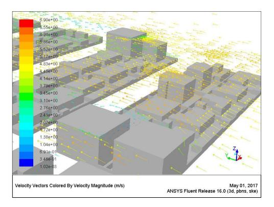
Figure 7.45 Wind path lines around buildings at height 10.5 m. [Author]
