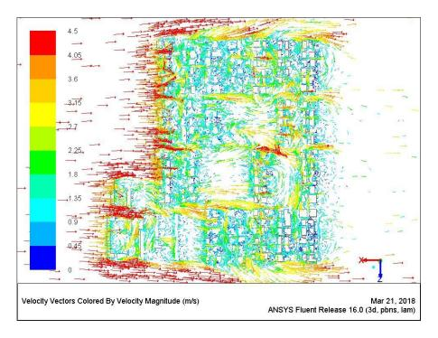
Figure 7.75 Wind pattern around buildings at a height of 1.5m [Author]
