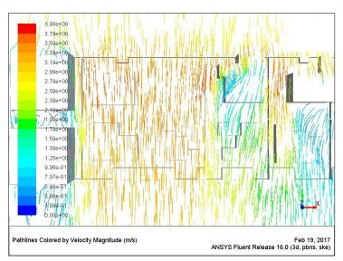
Figure 7.30 Wind pattern around buildings at a height of 10.5 m. [Author].
