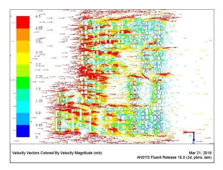
Figure 7.78 Wind pattern around buildings at a height of 7.5m [Author]
