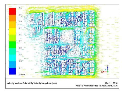
Figure 7.65Wind pattern around buildings at a height of 1.5m [Author]
