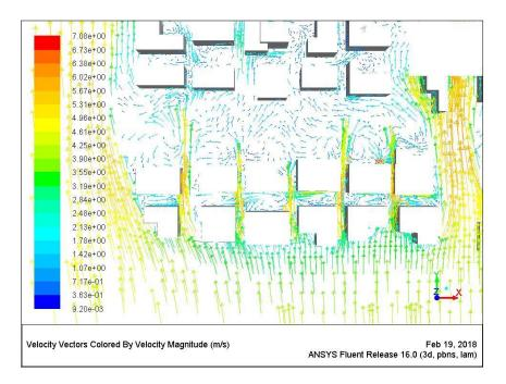
Figure 7.58 Wind pattern around buildings at a height of 7.5m [Author]
