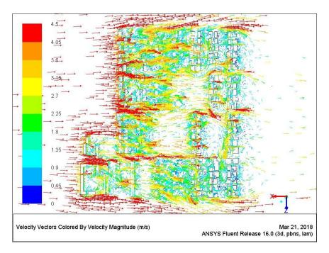
Figure 7.76 Wind pattern around buildings at a height of 4.5m [Author]
