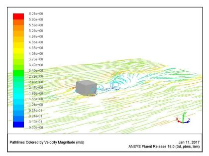
Figure 7-10. 3-D view for wind speed and direction. [Author]
