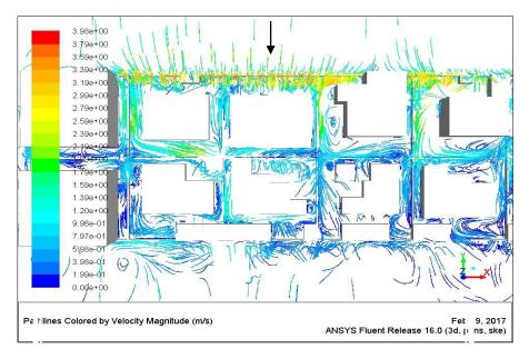
Figure 7.22 Wind pattern around buildings at 1m.
