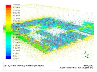
Figure 7.60Wind pattern around buildings at a height of 10.5m [Author]
