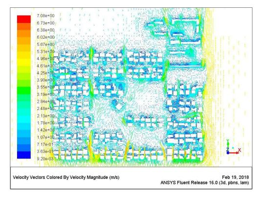
Figure 7.53 Wind pattern around buildings at a height of 4.5m [Author]
