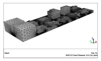
Figure 7.19 3D Tetrahedran mesh generated by Ansys 16 software. [Author].
