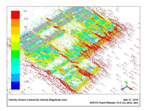
Figure 7.77 Wind pattern around buildings at a height of 4.5m [Author]
