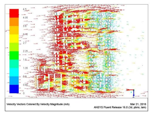
Figure 7.80 Wind pattern around buildings at a height of 10.5m [Author]
