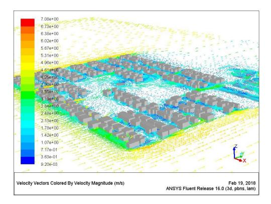
Figure 7.54 Wind pattern around buildings at a height of 4.5m [Author]
