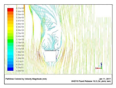
Figure 7.9 Wind pattern around the building (speed and direction) [Author]
