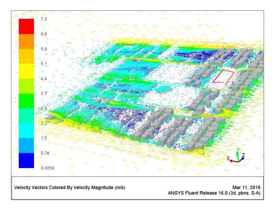
Figure 7.70 Wind pattern around buildings at a height of 7.5m [Author]
