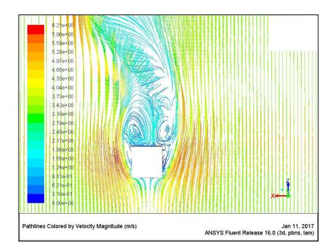
Figure 7.12 speed and direction of the wind around the building (mesh 0.1). [Author] After analyzing this model, the following findings have been reached:
