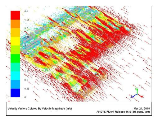
Figure 7.81 Wind pattern around buildings at a height of 10.5m [Author]
