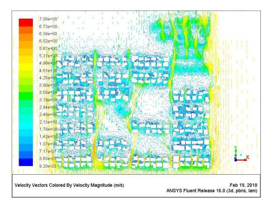
Figure 7.56 Wind pattern around buildings at a height of 7.5m [Author]
