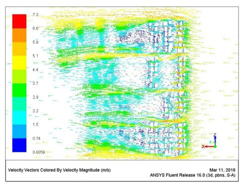
Figure 7.73 Wind pattern around buildings at a height of 10.5m [Author]
