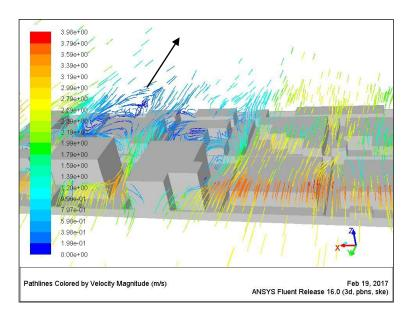
Figure 7.27 Wind pattern around buildings at a height of 4.5
