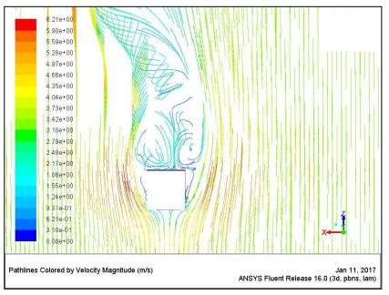
Figure 7.11 Speed and direction of the wind around the building (mesh 0.5). [Author] When the model was analyzed by using mesh with dimensions of 0.1, the results shown in figure 7.12 bellow was obtained and the following facts were noticed:
