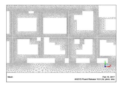
Figure 7.20 2D Tetrahedran mesh generated by Ansys 16 software. [Author].
