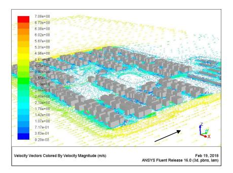
Figure 7.51 Wind pattern around buildings at a height of 1.5m [Author]
