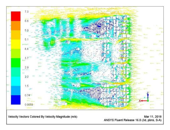
Figure 7.71 Wind pattern around buildings at a height of 7.5m [Author]
