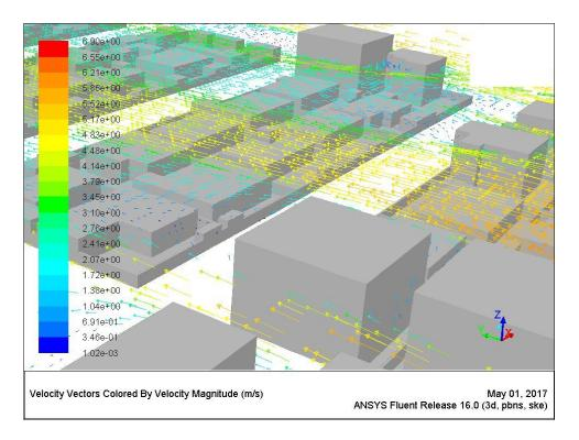
Figure 7.44 Wind path lines around buildings at height 10.5 m. [Author]
