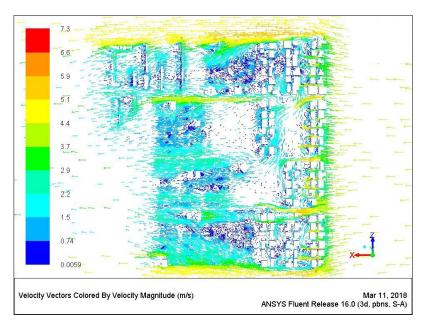
Figure 7.69 Wind pattern around buildings at a height of 4.5m [Author]
