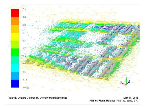
Figure 7.72 Wind pattern around buildings at a height of 10.5m [Author]
