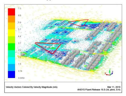
Figure 7.68Wind pattern around buildings at a height of 4.5m [Author]
