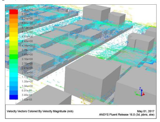
Figure 7-40 Wind path lines and speed around buildings at 4.5m. [Author]
