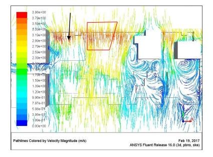
4-Wind speed in internal courtyards ranges between 2m/s to 3m/s.
