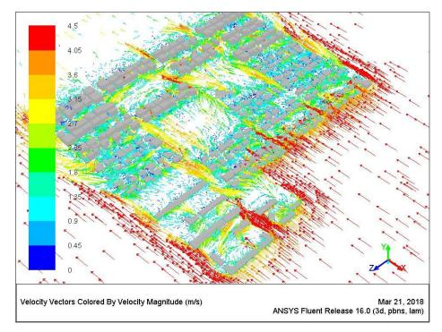
Figure 7.74 Wind pattern around buildings at a height of 1.5m [Author]
