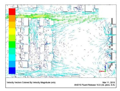
Figure 7.67 Wind pattern around buildings at a height of 1.5m [Author]
