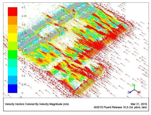
Figure 7.79 Wind pattern around buildings at a height of 7.5m [Author]
