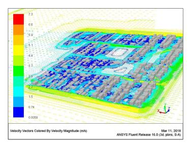
Figure 7.66 Wind pattern around buildings at a height of 1.5m [Author]
