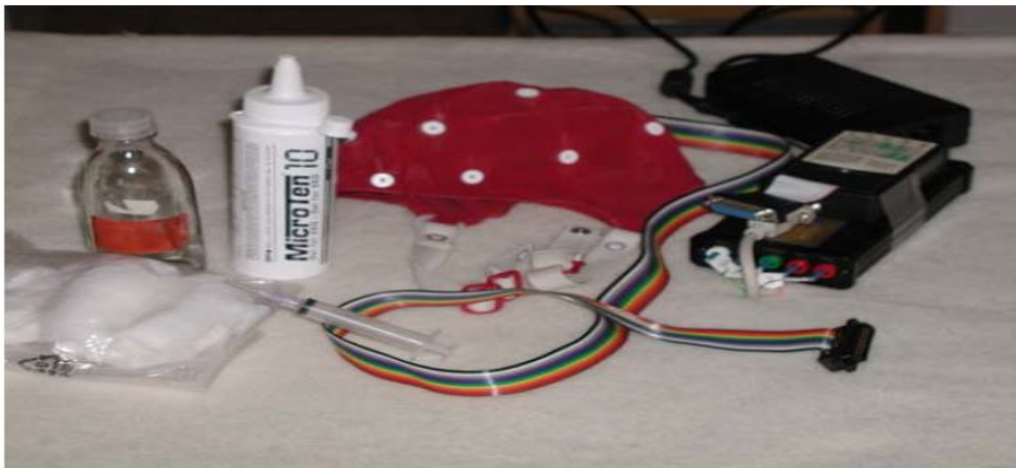
Fig(3.3). Equipment for EEG recording: amplifier unit, electrode cap, conductive jelly, injection, and aid for disinfection.
