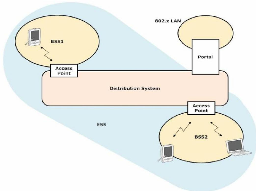
Figure 2-3: WLAN Infrastructure based architecture
