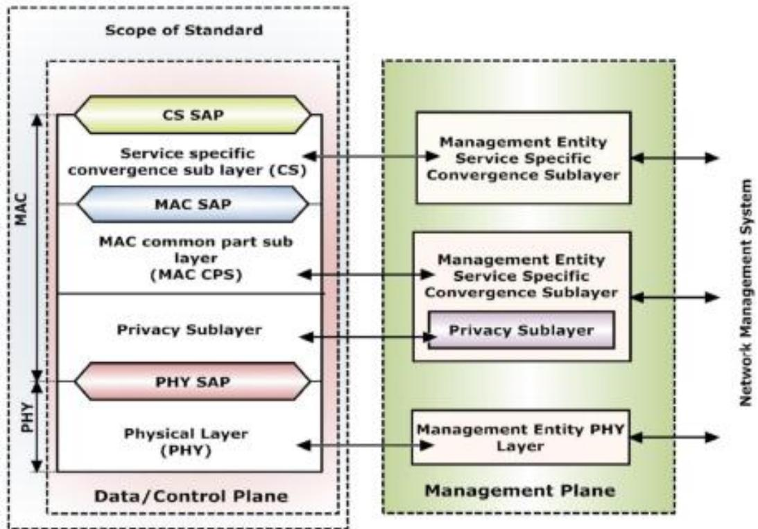
Figure 2-1: NETWORK Reference model of IEEE 802.16
