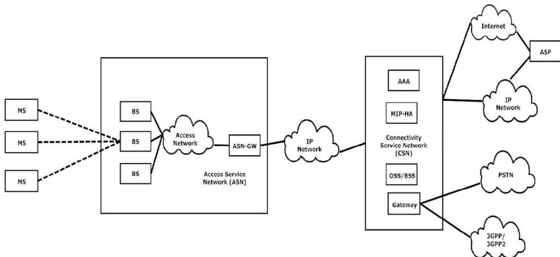
Figure 2-2 WiMAX Network Architecture
