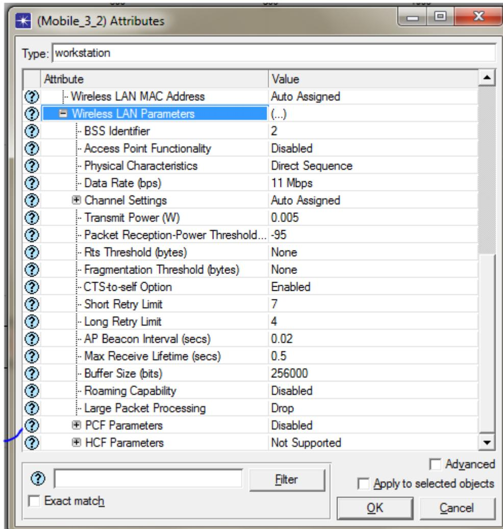
Figure 3-6: WLAN subscriber station parameters
