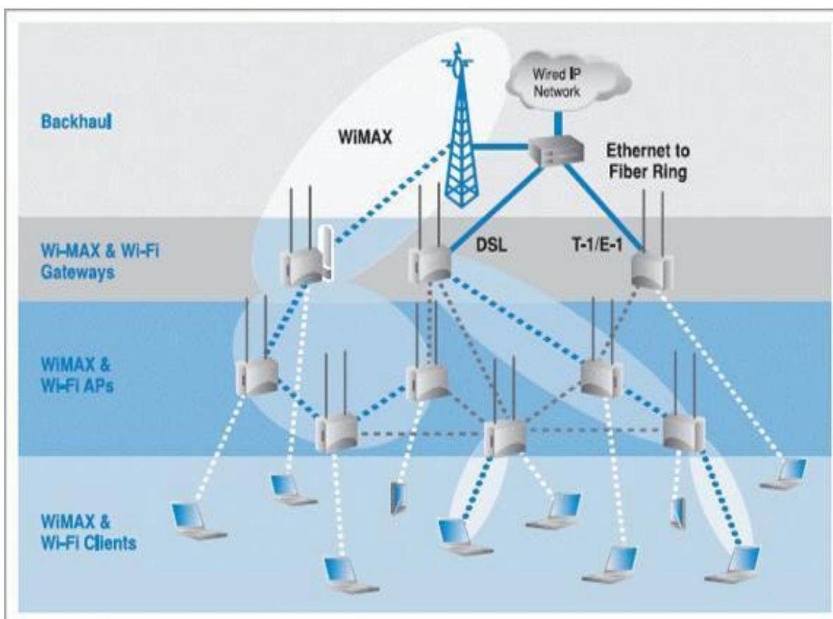
Figure 2-6: Wi-Fi –WiMAX Fully Integrated Architecture
