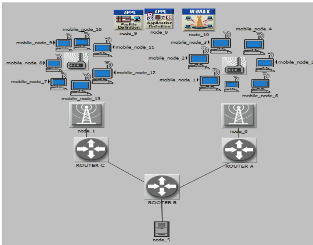
Figure 3-7: Network Model for WiMAX-WLAN Integrated Network
