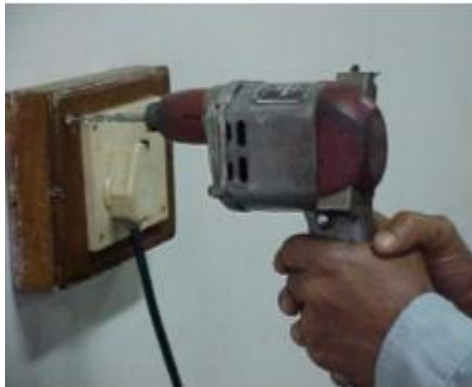
Fig. 2.7 Hand Drill in Operation
