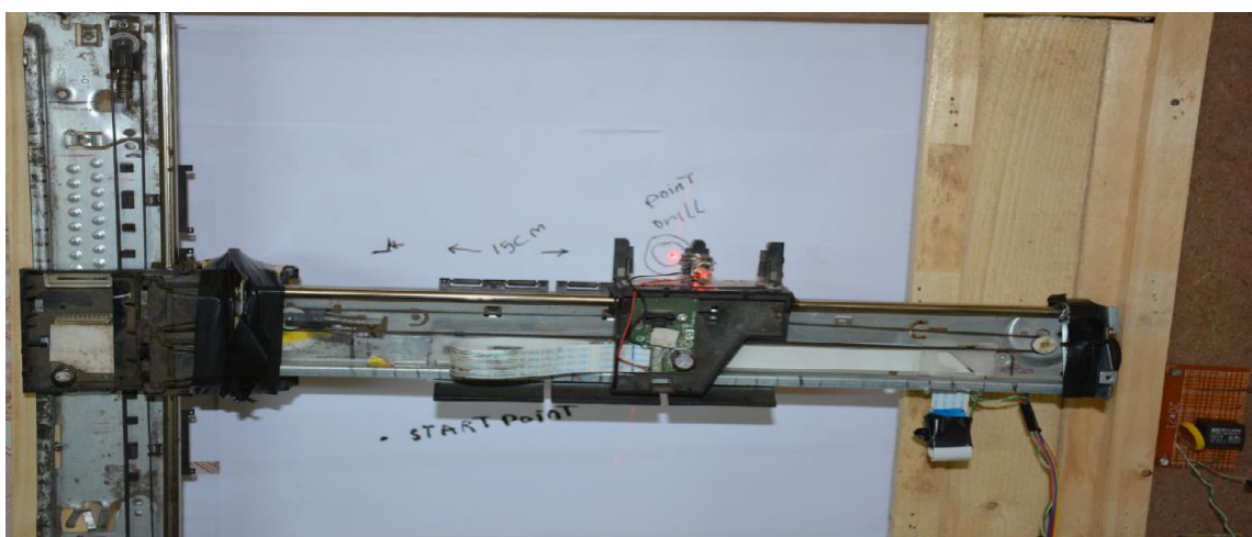
Fig 4.3 Laser drilling machine running
