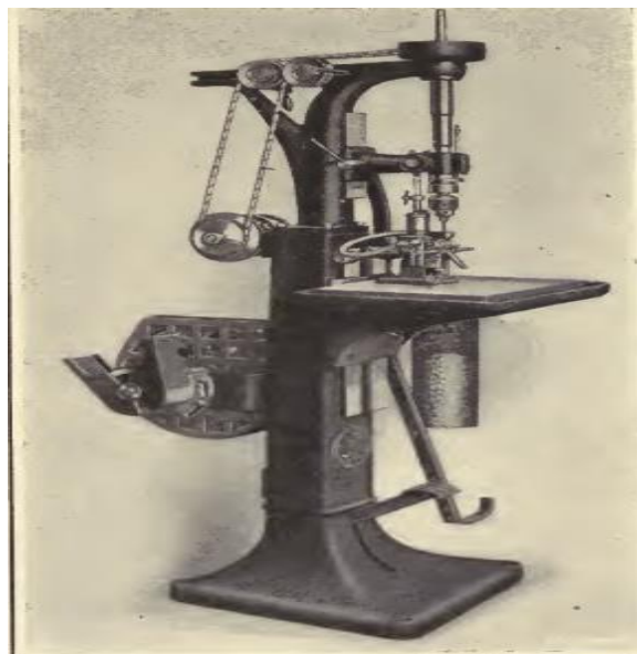
Fig. 2.2 Sensitive drilling machine with special jig for drilling cross holes in pins
