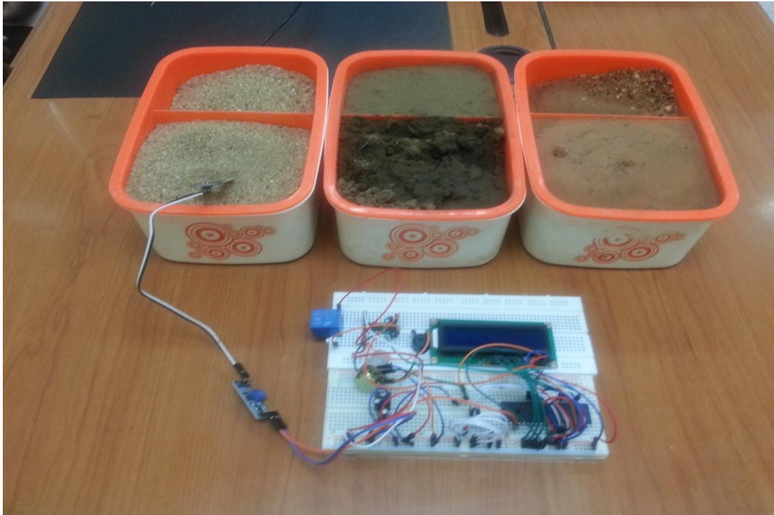
Figure 4.1: Reading sensor values from sand, loam and red soil
