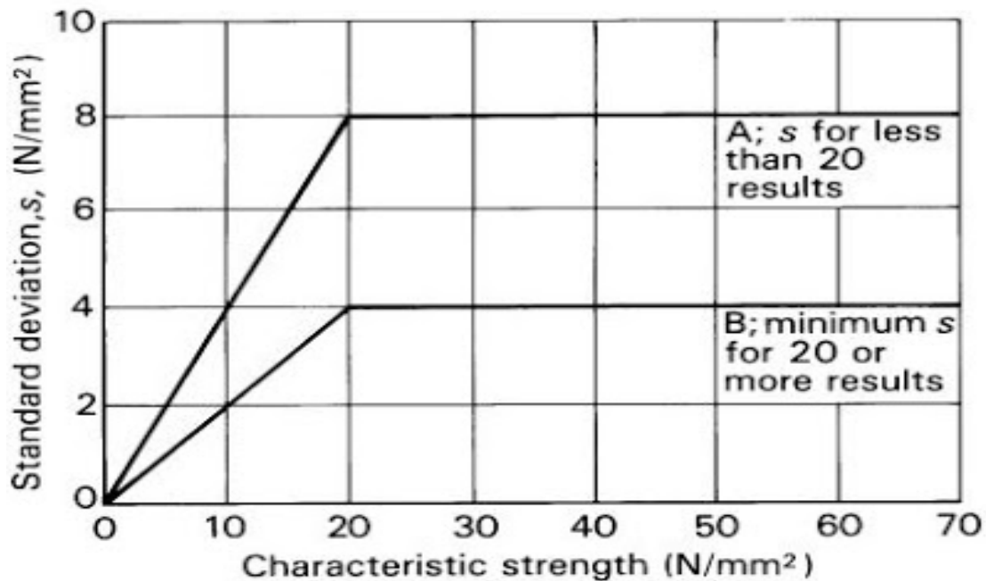
Figure (3.5): Relationship between standard deviation and characteristic strength.
