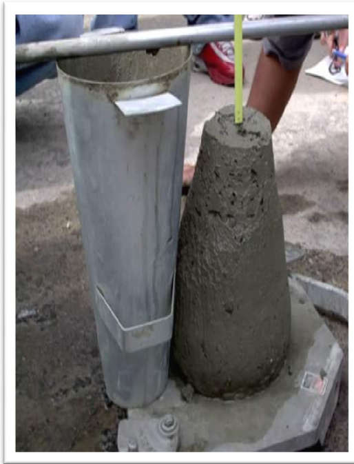
Figure (4.13): Slump Test
