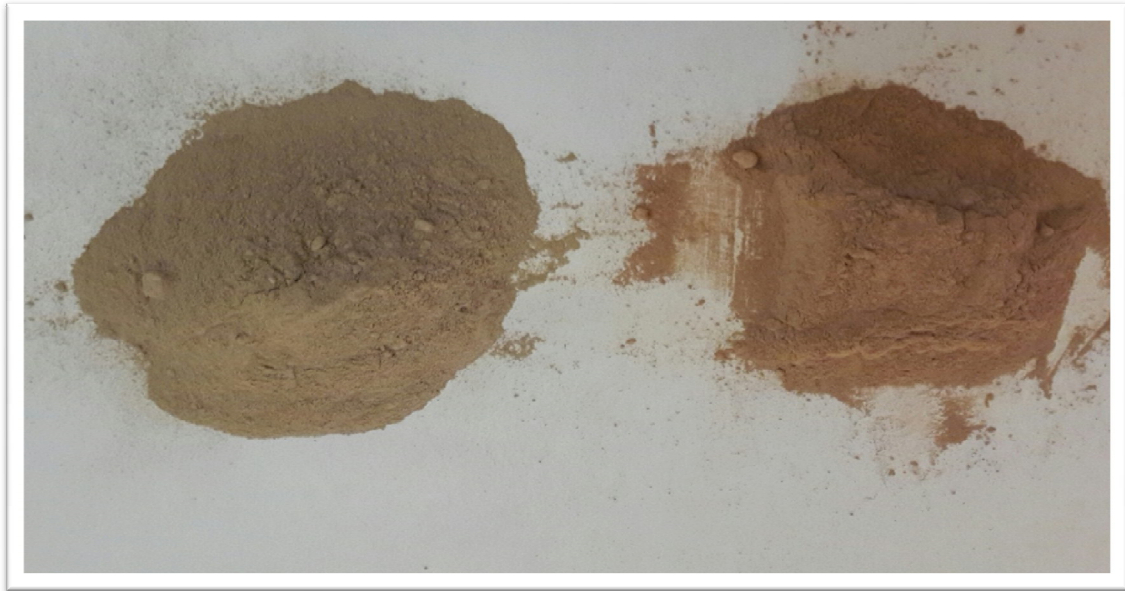
Figure (4.11): Ceramic Waste Powder before & after Treated
