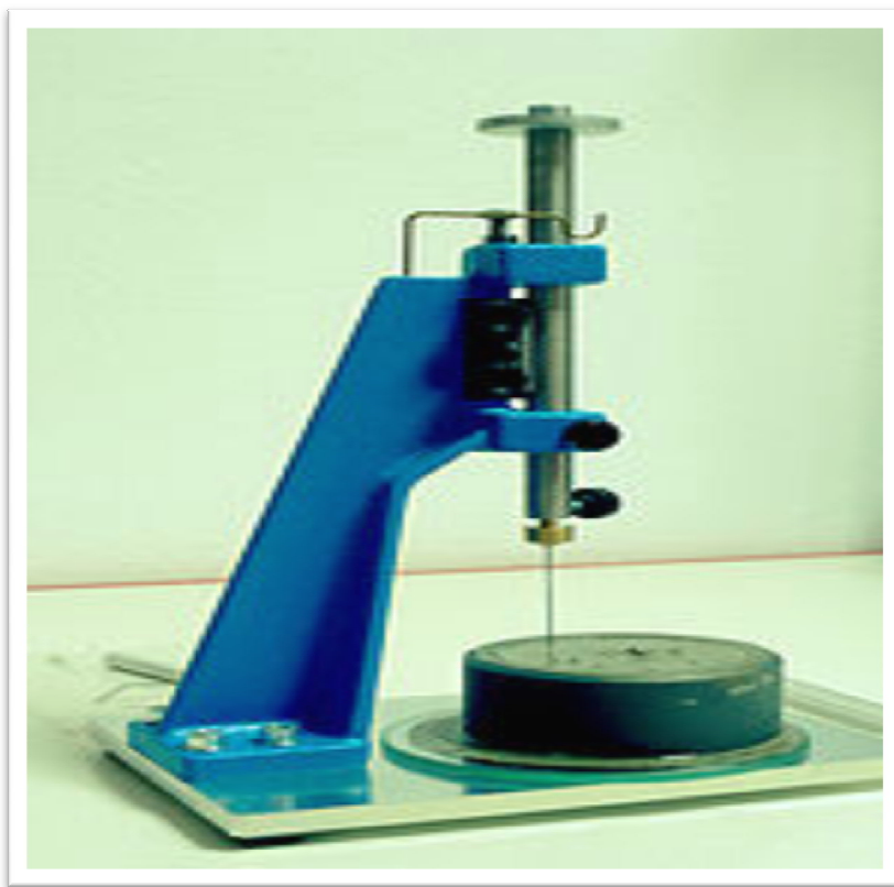
Figure (4.2):Vicat Apparatus
