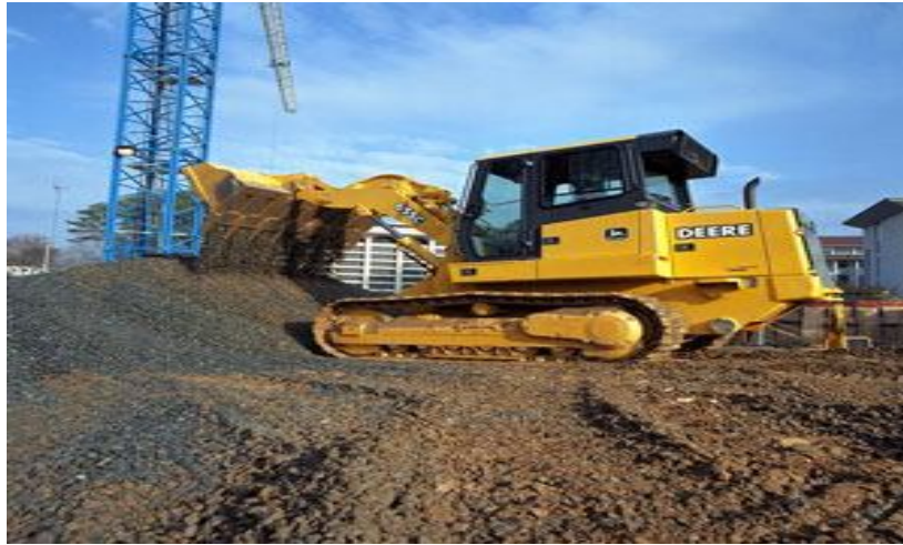
Fig.(2-8): Typical type of crawler loader
