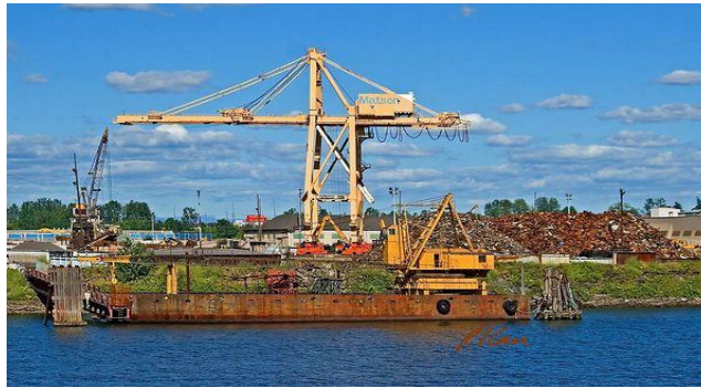
Figure 2.10: Rail mounted tower crane.
