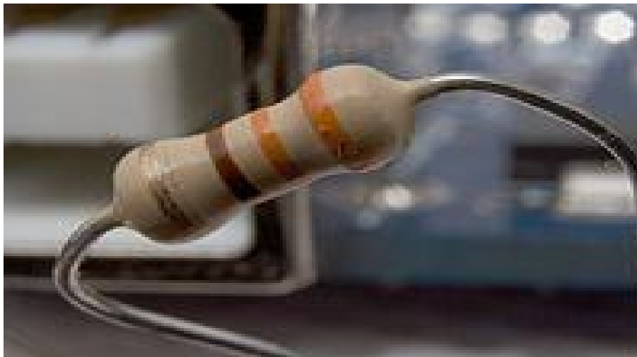
Fig.4.1. resistor is a passive two-terminal electrical component. [17].
