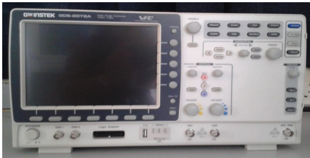
Fig 4.8. GW Instek digital oscilloscope with wide frequency range.
