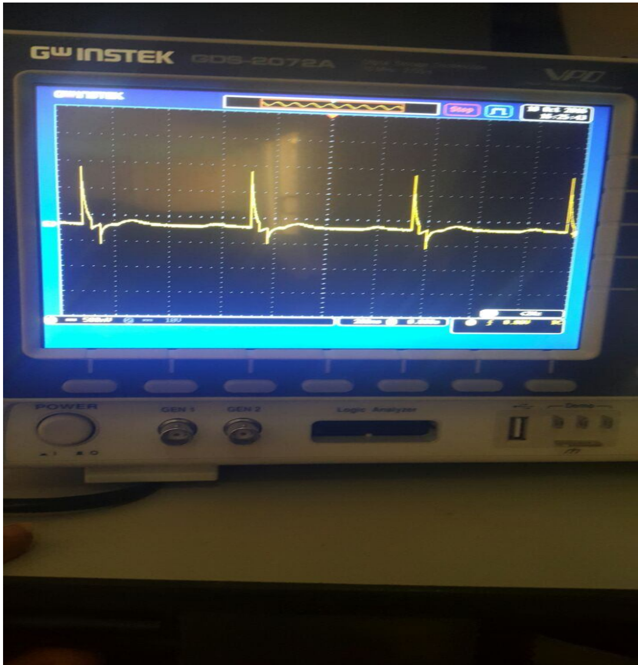
Fig 5.3.The output of the final simulator circuit (hardware) shown using an oscilloscope with scale 500m V.
