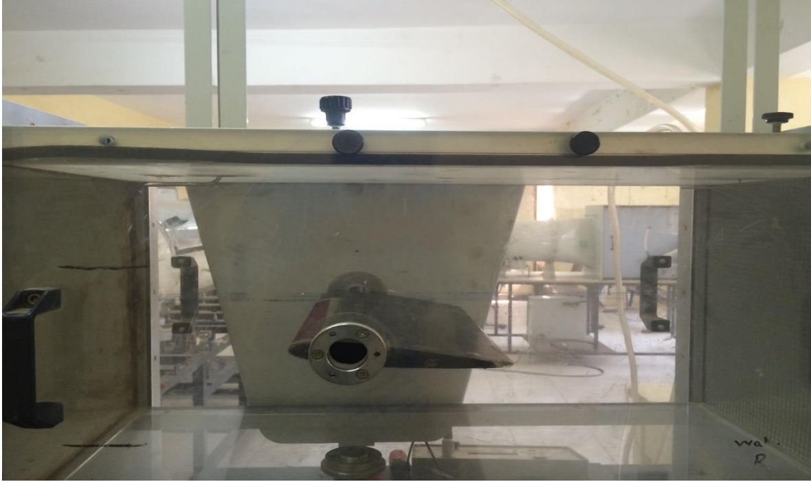
Figure 11: Blade within rough surface in the wind tunnel
