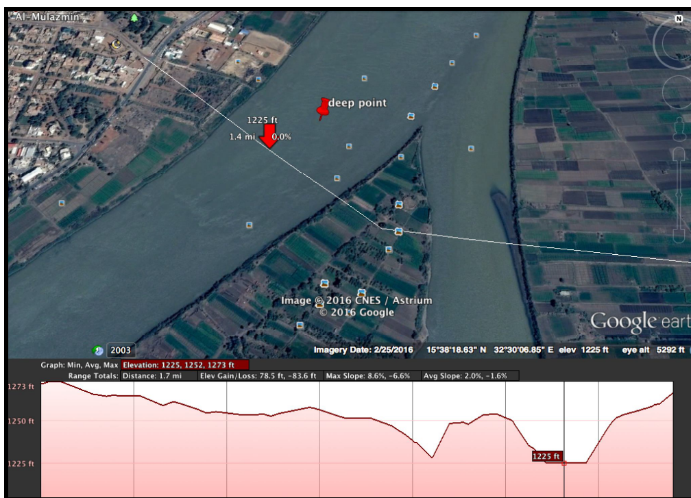
Figure 4-9 Maximum Depth of Water at Track Area
