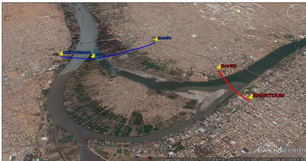
Fig 3-14 the Proposed Tunnel Tracks
