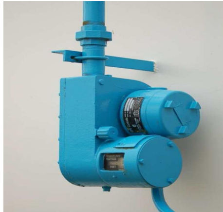
Figure 4.9 measurement head of a spring-reel tape-and-float liquid level transmitter
