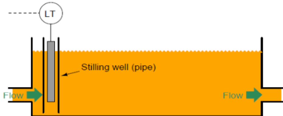
Figure 4.24 liquid level measurements with stilling well
