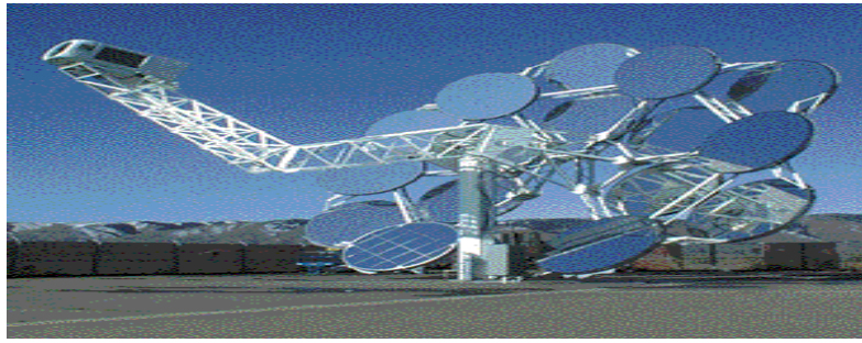
Figure (2.9) Parabolic Dish Collector With a Mirror-like Reflectors And an absorber at the focal point [Courtesy of SunLabs - Department of Energy] .
