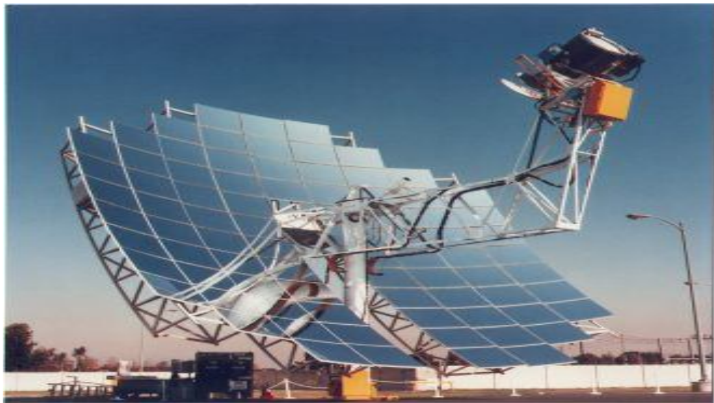
Figure (2.10) Solar Dish Stirling Engine .
