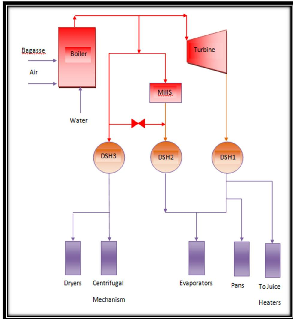
**Figure 3.1** Flow diagram of Elgunied Sugar Factory power plant
