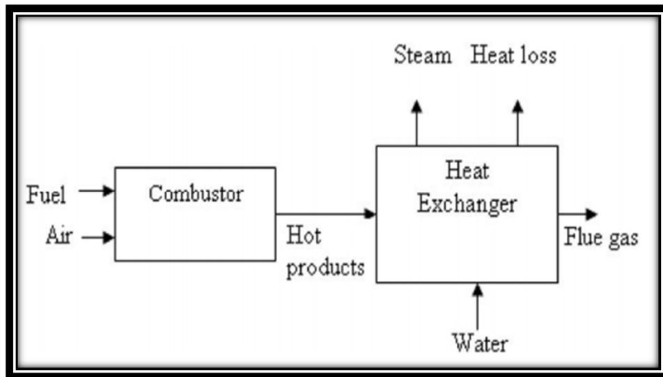
**Figure 3.2** Schematic diagrams of combustor and heat exchanger in a boiler
