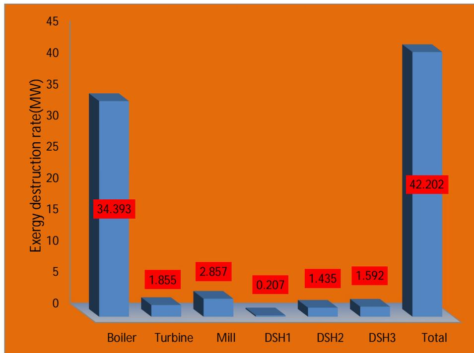
**Figure 4.1.a** Exergy Destruction Rate (MW) of Components
