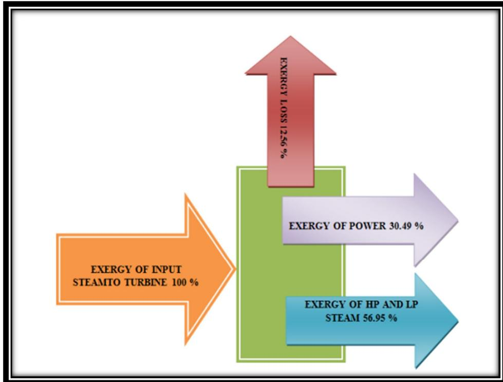
**Figure 2-2** Diagram for Exergy Flow Through Steam Turbine At 85 %MCR [19]
