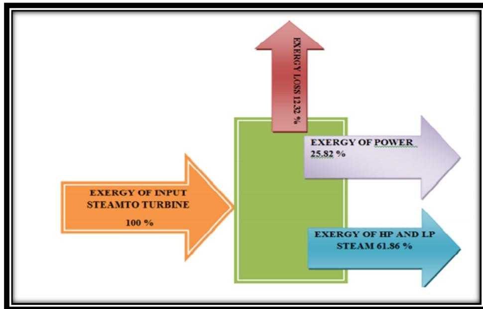
**Figure 2.1** Diagram For Exergy Flow Through Steam Turbine At 70 %MCR [19]
