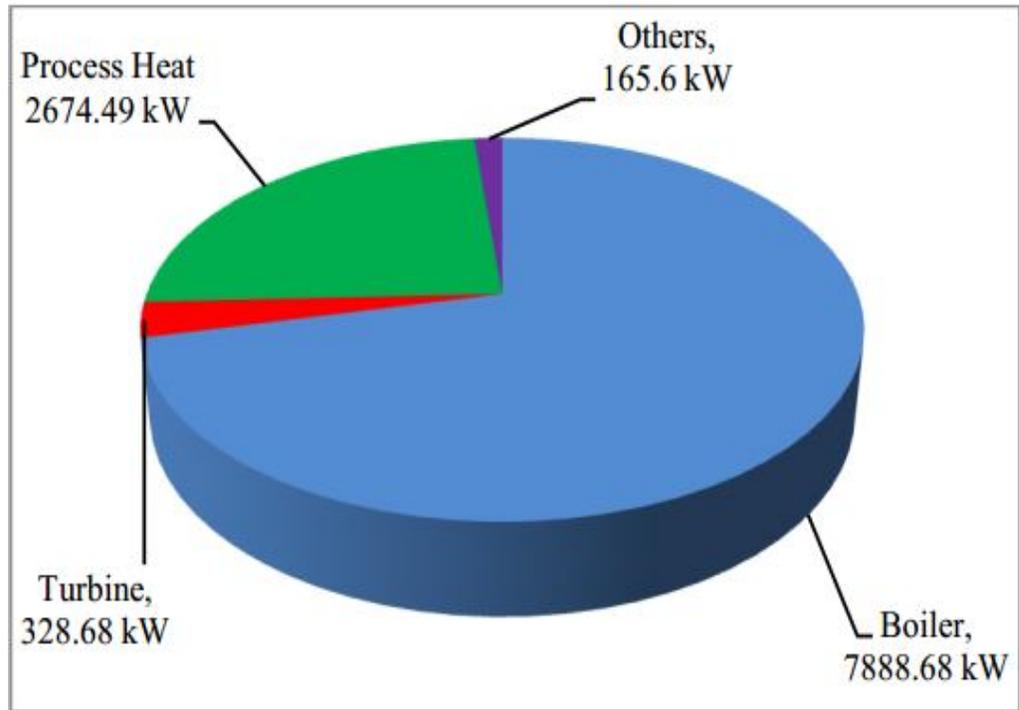
**Figure 2-3** Exergy destruction in simple back pressure cogeneration plant [2].
