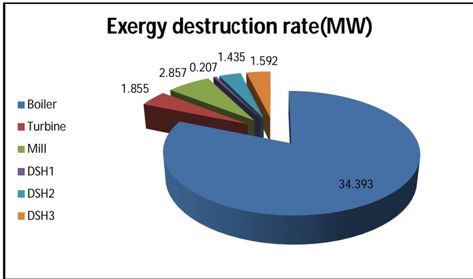
**Figure 4.1.b** Exergy Destruction Rate (MW) of Components
