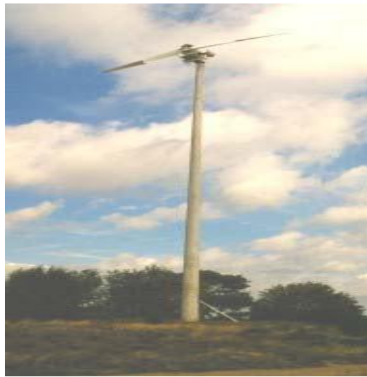
Figure 2.5: 2-blade HAWT,30 kW, Pitch Wind Systems AB Company (Sweden).
