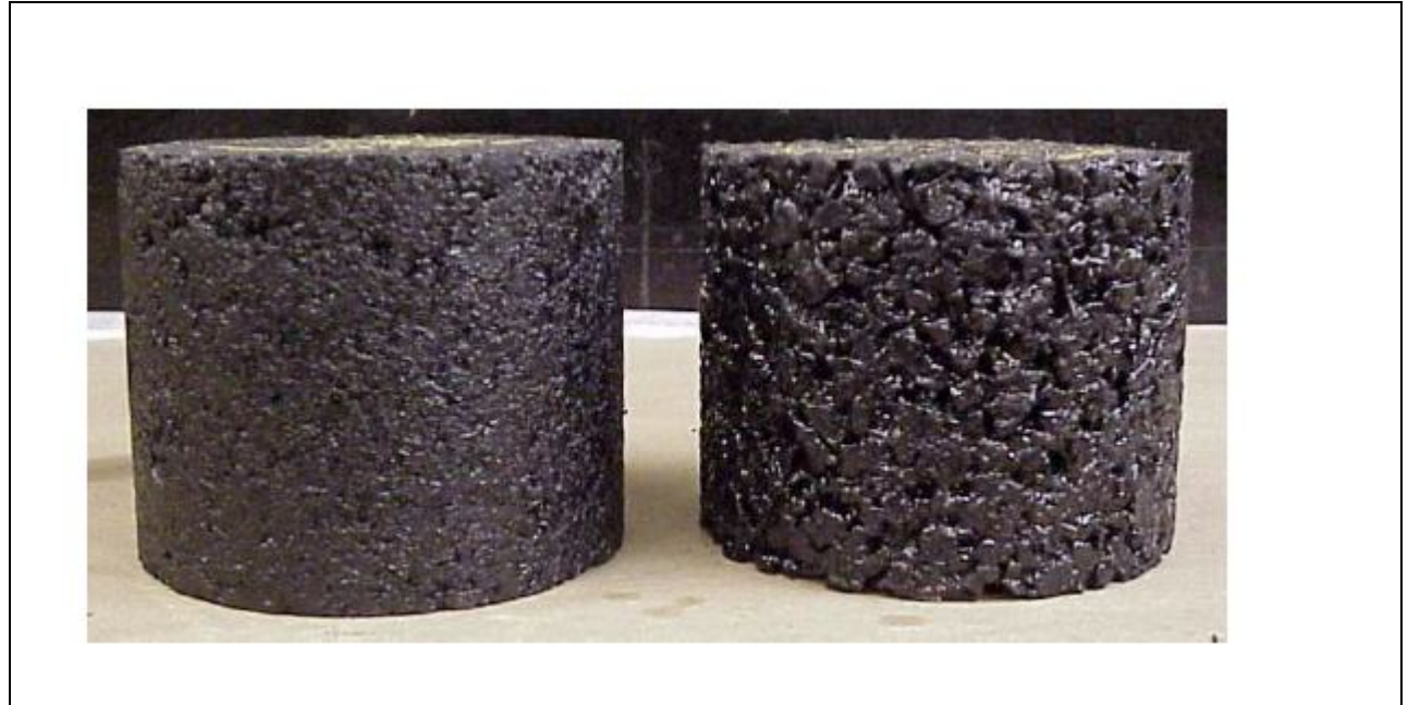
Figure 2.3: Dense Graded HMA (Left) VS SMA (Right)
