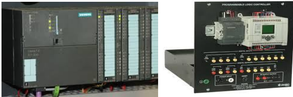
Figure 2.5 Programmable logic controller.
