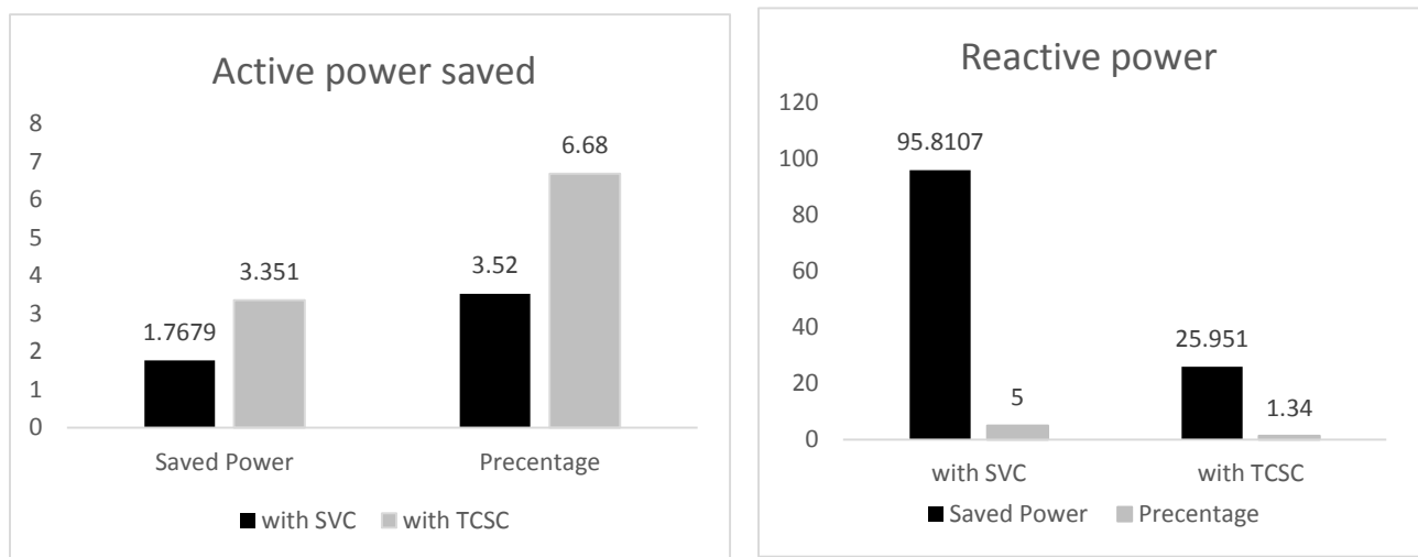
Figure 4.18: Total active & reactive power Losses without and with FACTS
