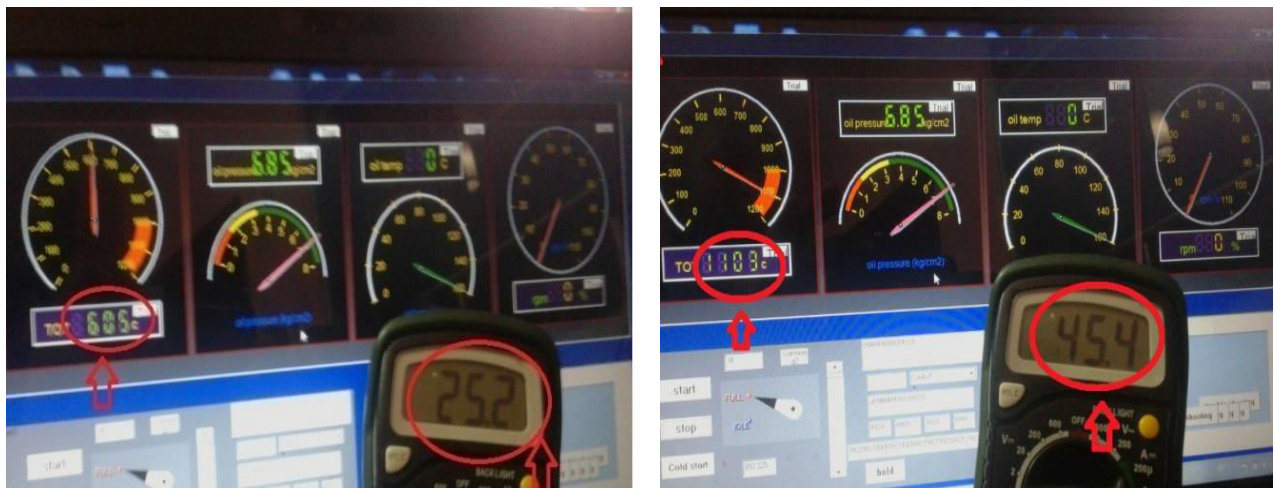
Figure (5.4) Gas temperature indicator calibration process
