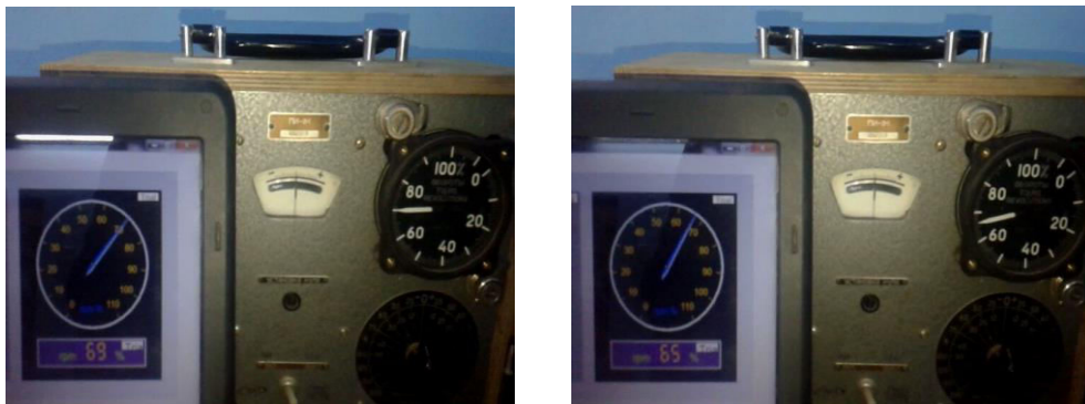
Figure (5.2) Tachometer calibration process
