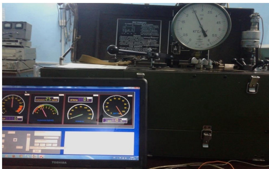
Figure (5.6) Oil pressure testing unit
