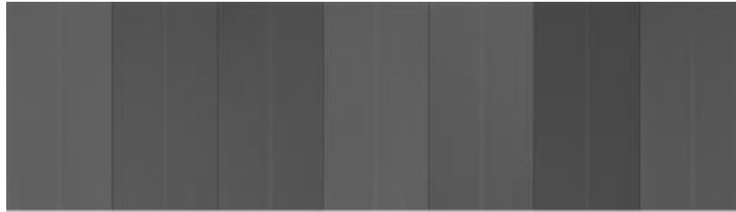
Figure (2.6) Offset image of a 7-panel detector (RadEye7H). It can be seen that each panel has different dark current average from one another; the highest (light) is from the left of the first and 4 panel, while the lowest (dark) is in the sixth panel ( oftankonyv.reak.bme.hu ).
