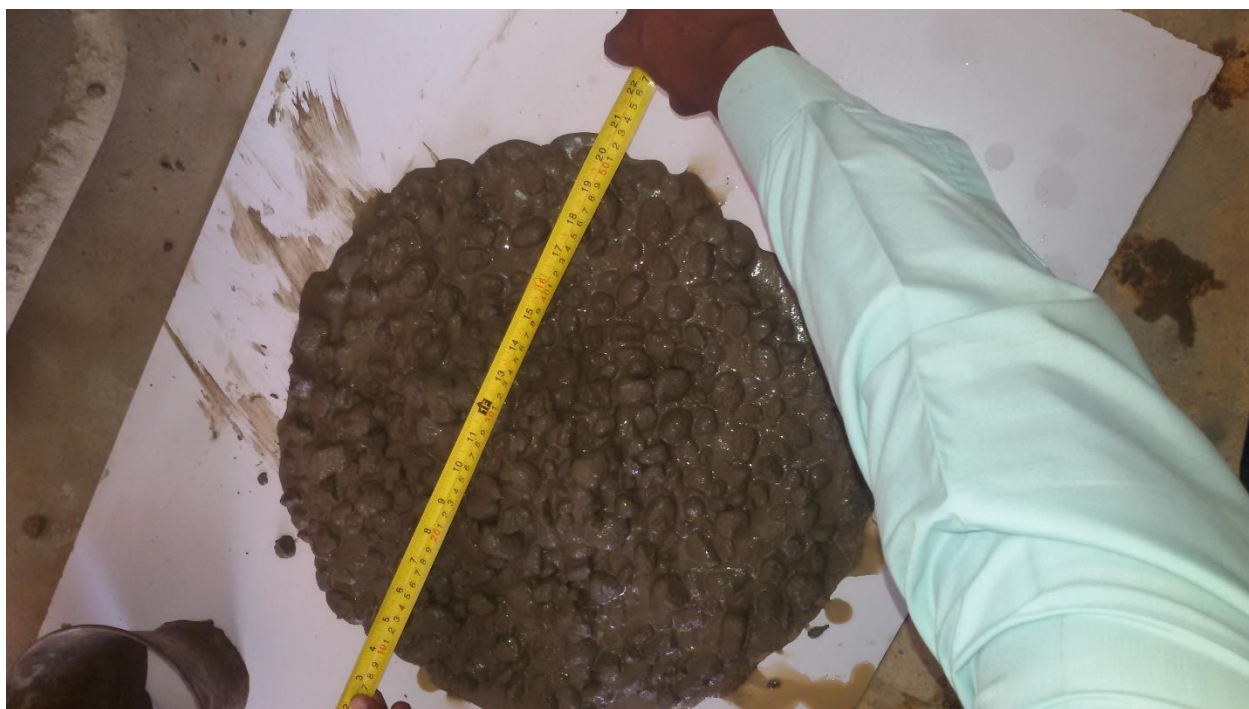
Appendix (E.4)b: measure of diameter in other direction
