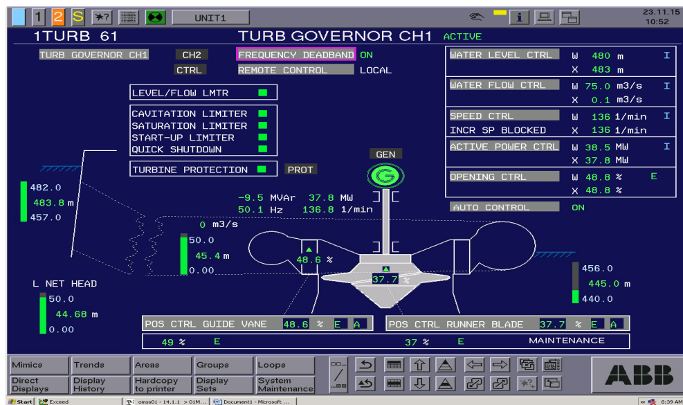
Figure 3.5.C unit 1 turbine governor channel [8]
