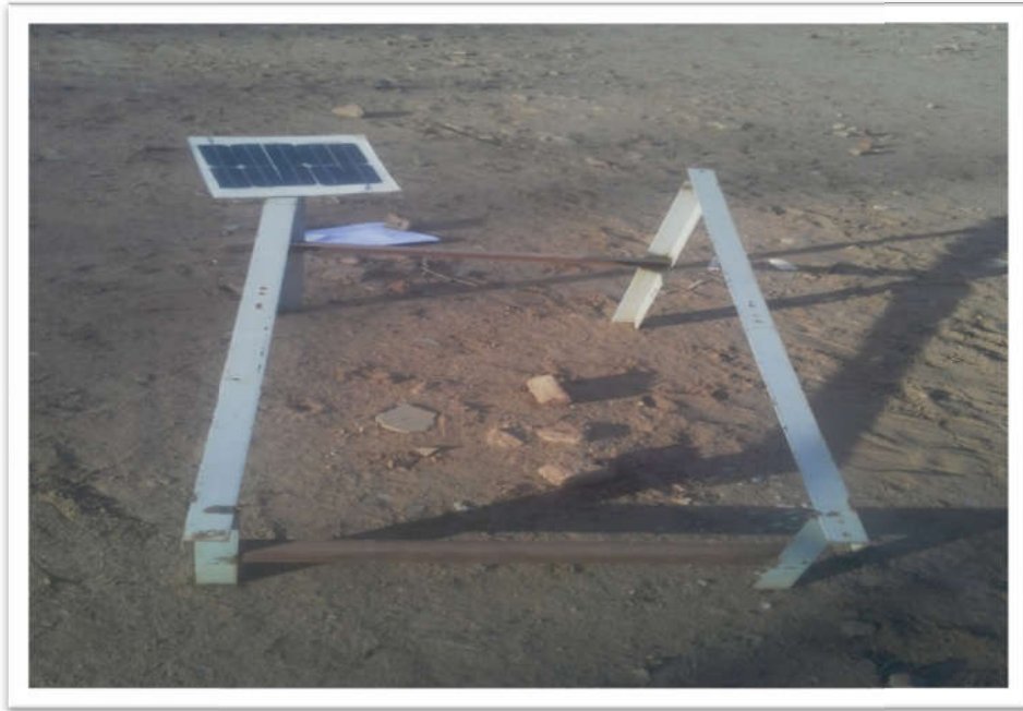
Figure 4.1 fixed SobaSolar PV module with acrylic glass cover
