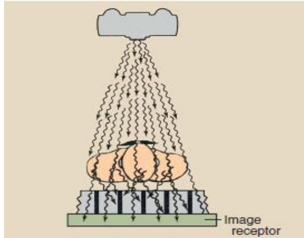
Figure(2.3) Radiographic grid absorbed scattered x-rays radiation from the patient.
