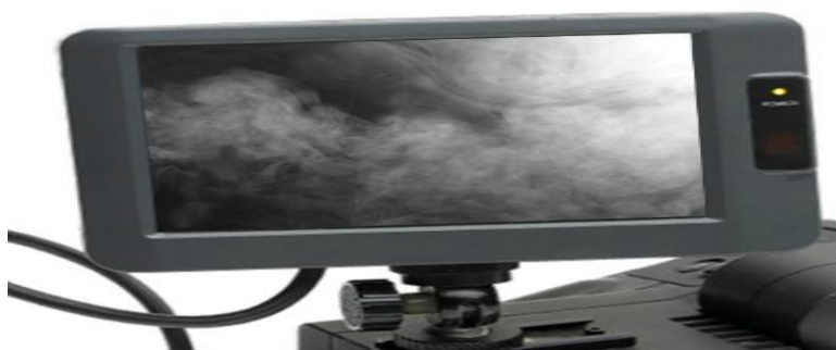
Figure 3.21: Gas leakage occurred in infrared camera as smoke
