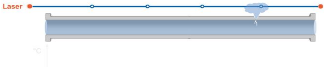
Figure 3.15: The cable installed above gas pipeline
