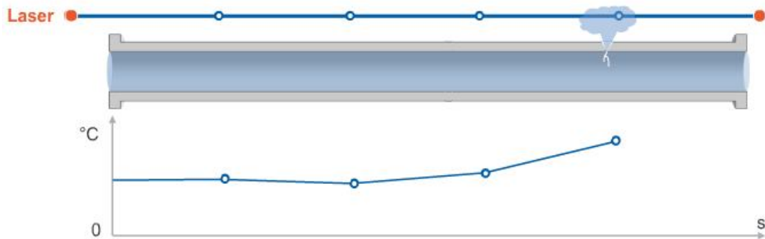
Figure 3.14: Temperature profile against reflected pulses
