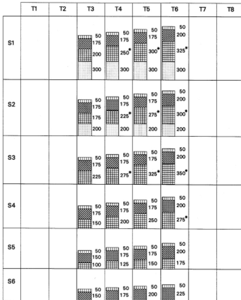
Note: 1 \* Up to 100mm of sub-base may be substituted with selected fill provided the sub-base is not reduced to less than the roadbase thickness or 200mm whichever is the greater. The substitution ratio of sub-base to selected fill is 25mm : 32mm.
