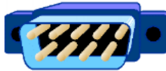
Figure2.9: The DB-9 connector used for the serial ports of IBM PC computers.
