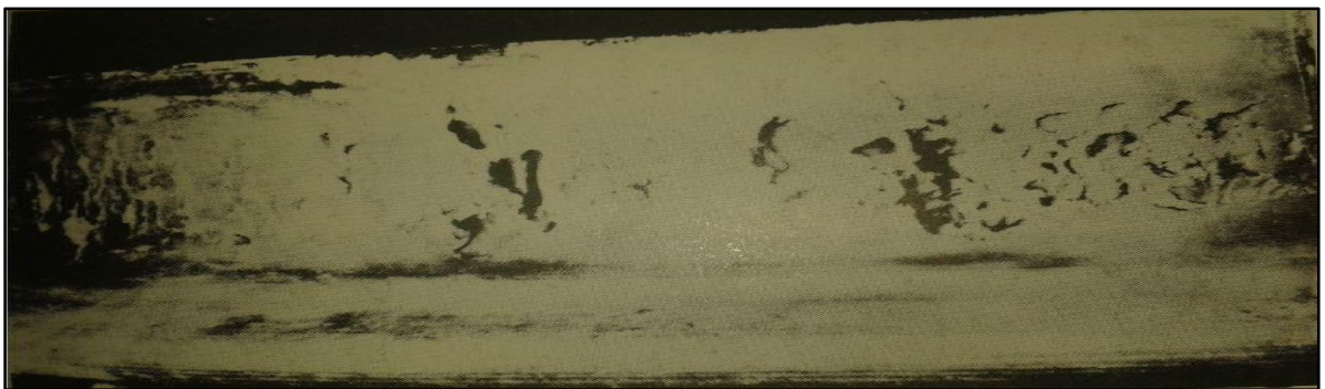
Fig (2.21) shelling of wheel tread due to excessive loading.
