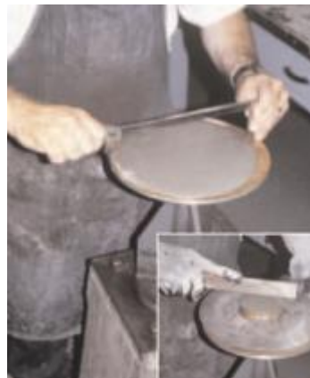
Figure (2.4): Consistency test for mortar using the flow table. The mortar is placed in a small brass mold centered on the table (in-set).
