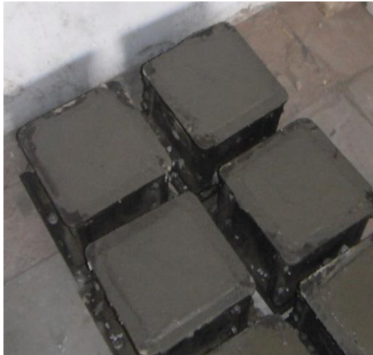
Figure (3.4): Typical concrete cubes.
