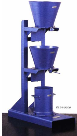
Figure (2.11): Compacting Factor apparatus.
