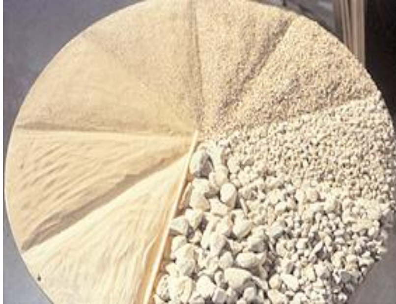
Figure (2.7): Range of particle sizes found in aggregate for use in concrete.
