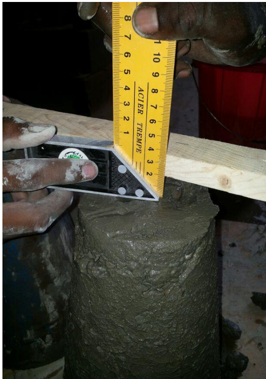
Figure (3.2): Slump test.
