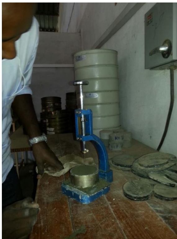
Figure (3.1): Setting time test.
