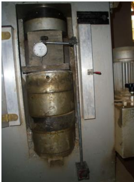
Figure (3.3): Axial deformation test.
