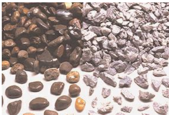
Figure (2.6): Coarse aggregate. Rounded gravel (left) and crushed stone (right).
