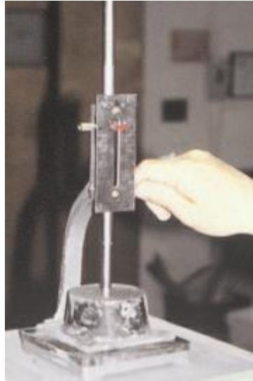
Figure (2.3): Normal consistency test for paste using the Vicat plunger.
