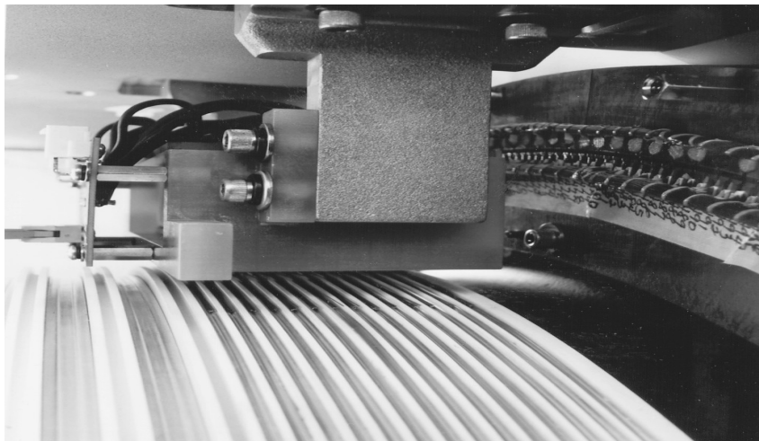
Figure 2.6 Slip ring in CT machine
