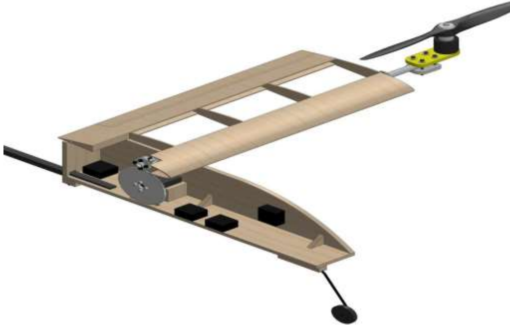
Fig. (3.9): Cross section view of tilt mechanism
