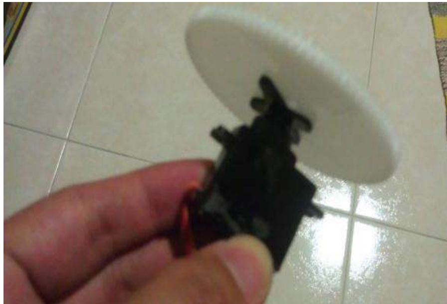
Fig. (3.8): Spur Gear attached to servo
