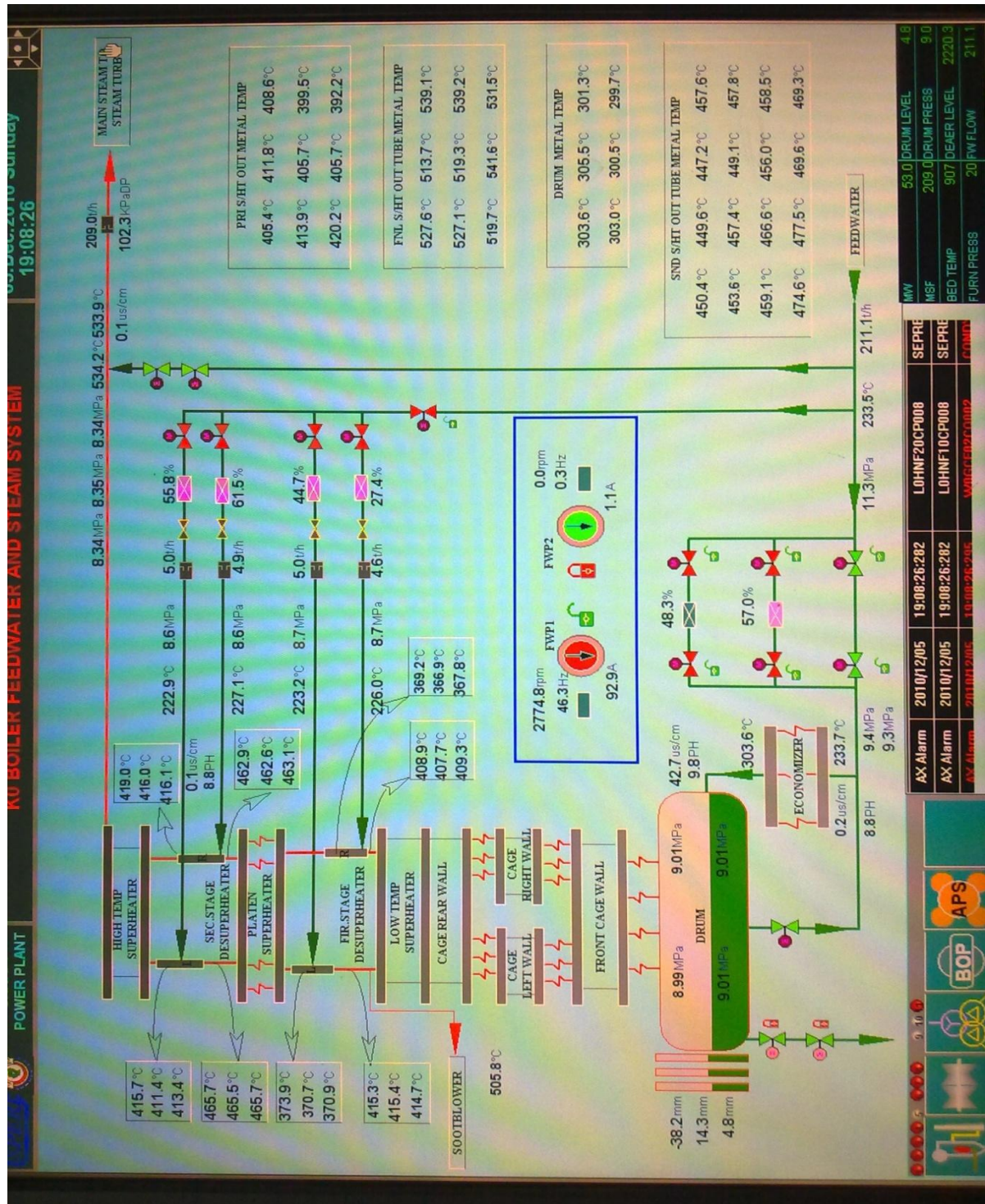
Figure 3.1: Steam superheat temperature control process description
