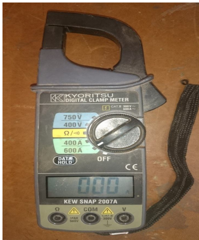
Figure 4.3: Digital Clamp Meter Device to Measure the Loads
