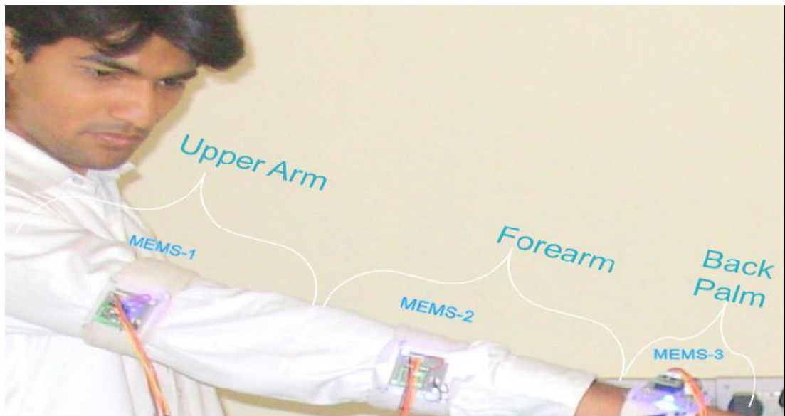
Figure 2.10: Placement of Sensors Robotic Arm
