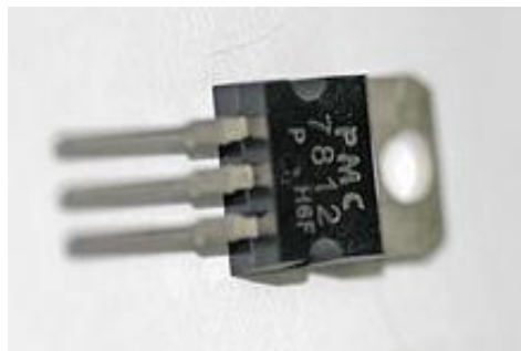
Figure2.25 A popular three pin 12 V DC voltage regulator IC.
