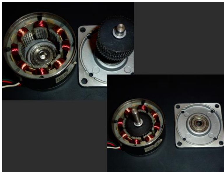
Figure3.6: A bipolar hybrid stepper motor
