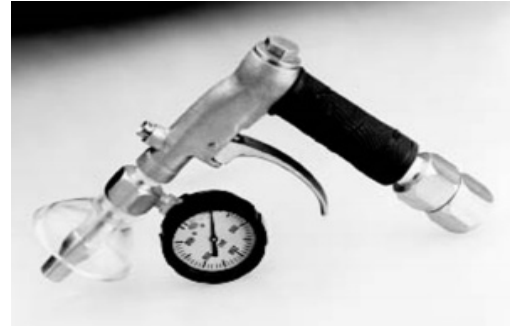
Fig(4.6)Water gun for brushes and scraper
