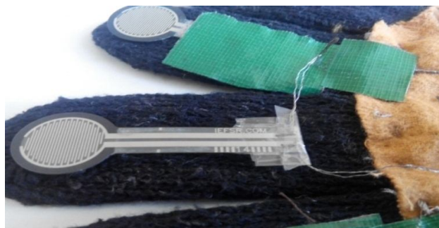
Figure (6.1): Replacing metal terminal with conductive thread
