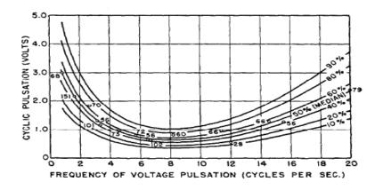
Fig [2.2] cyclic pulsations of voltage at which flicker of 115-volt tungsten filament lamp is just perceptible.
