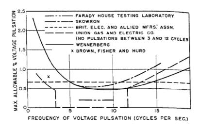
Fig [2.5] recommended maximum allowable cyclic variation of voltage.
