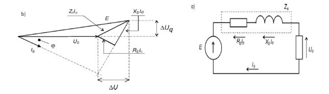
Fig [2.1] per phase equivalent circuit of supply net work (a)And phasor diagram for resistive-inductive load E≥Vo (b)
