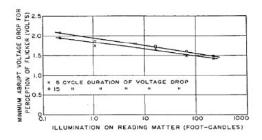
Fig[2.3] -Minimum abrupt voltage drop for perception of flicker of 60-watt, 120-volt coiled-coil tungsten-filament lamps.
