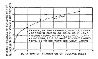
Fig [2.4]: Effect of duration of transition of voltage on average Threshold of perceptibility of flicker of tungsten-filament lamps.
