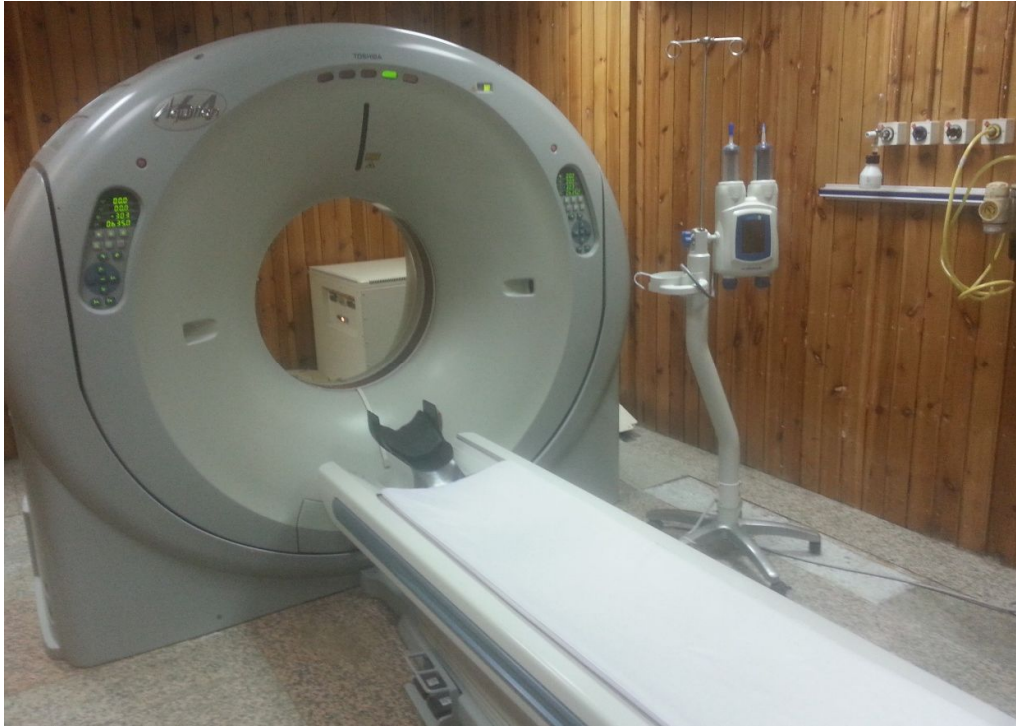
Figure 3-2: CT machine in Military hospital (Toshiba Aquilion 64 slices).
