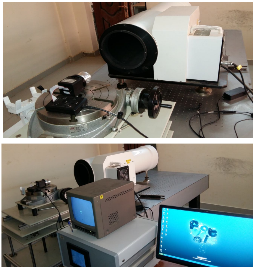
Figure (3.7): The MRTD test station and thermal camera
