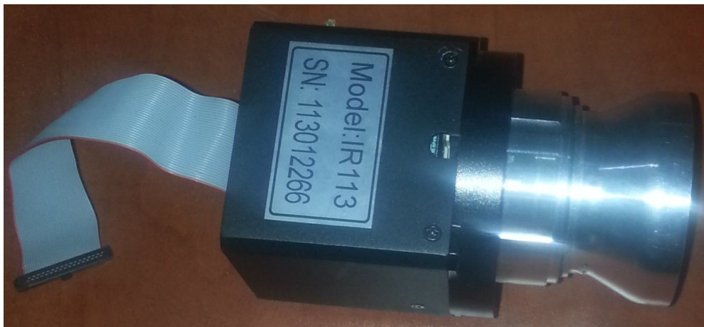
Figure (4.13): The thermal camera [Intended thermal camera here: the integration between the designed and fabricated IR optical system (lenses) and the detector module (IR113) which was selected by using the designed and manufactured mechanical case]
