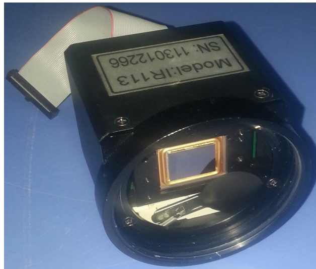
Figure (4.11): Thermal detector module (IR113) inside his mechanical case
