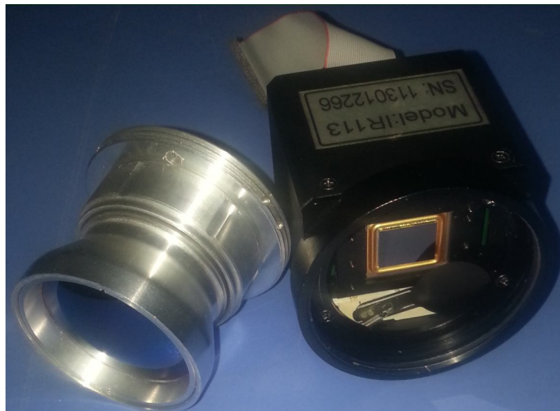
Figure (4.12): Assembly of the optical system (3 lenses) on mechanical case, and thermal detector module (IR 113)
