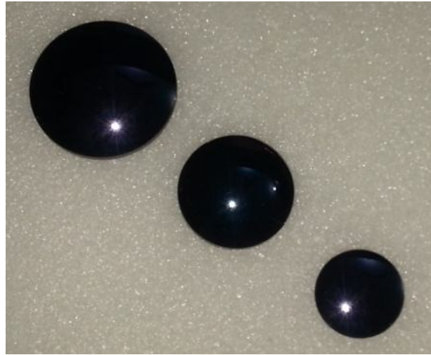
Figure (4.10): Real picture of IR optical system (3 germanium lenses) after manufacturing
