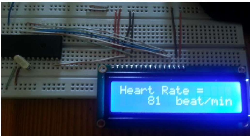
Figure 6.1: the pulse rate displaying for the first case
