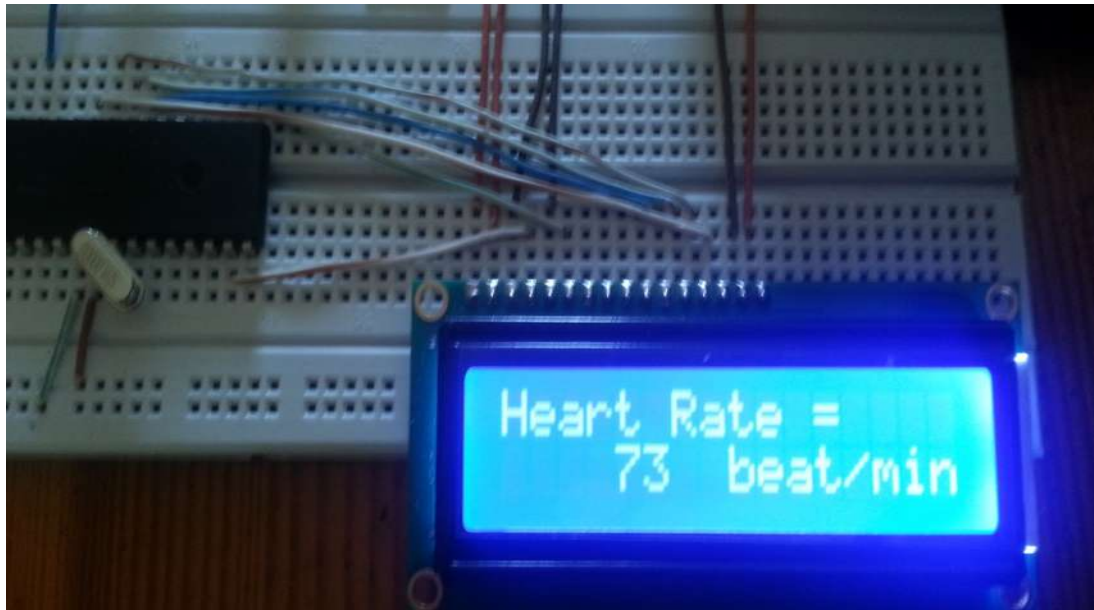
Figure 6.3: the pulse rate displaying for the third case
