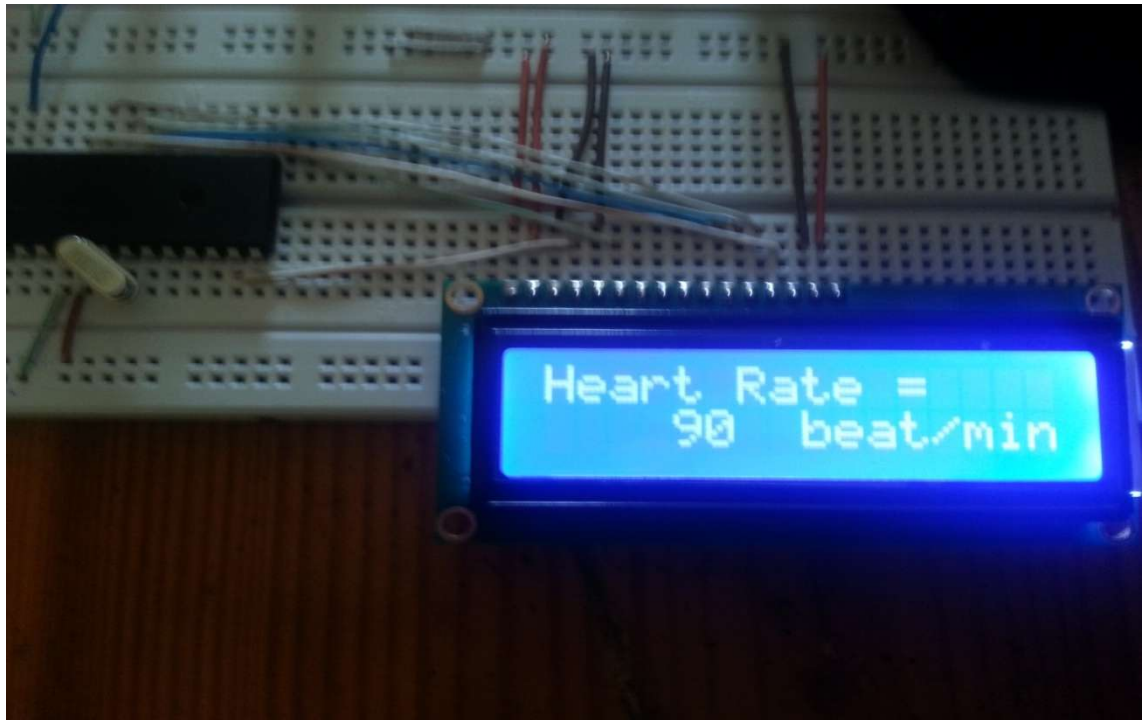
Figure 6.7: the pulse rate in practical circuit
