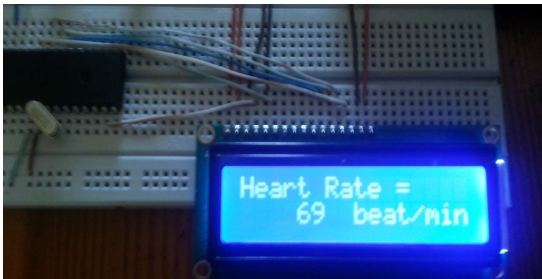
Figure 6.4: the pulse rate displaying for the fourth case
